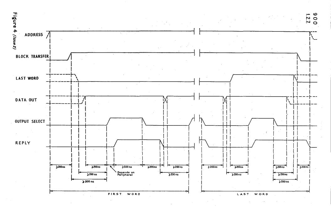
900 series INTERFACE BLOCK OUTPUT TIMING
